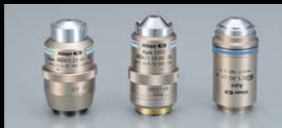
CFI Apochromat 40xWI \lambda S, NA1.25 (left) CFI Apochromat LWD 40xWI \lambda S, NA1.15 (middle) CFI Apochromat 60x Oil \lambda S, NA1.4 (right)
