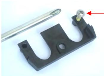
← Cut the thread with the enclosed screw
