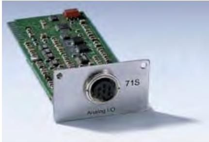
Analogue Module (LAUDA catalogue no. LRZ 912) has two inputs and two outputs, which are brought out to a six-pole DIN socket to Namur Recommendation (NE28).
