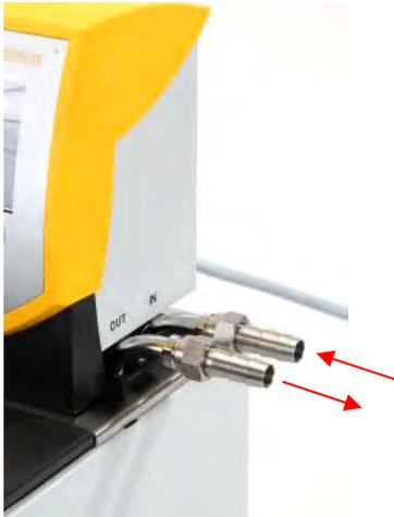
To ensure the greatest volume flow, with operation as a circulation thermostat ensure the shortest possible hose connections with the largest possible hose internal diameter.
