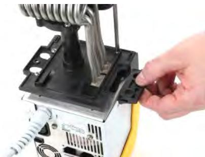
The pump connection set can be mounted on one side of the control head (see illustration).
