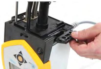
The cooling coil can only be mounted on one side of the control head. This is located on the side with the mains switch.
