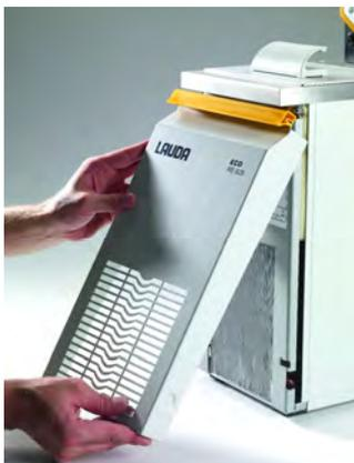
The cooling circuit is largely maintenance-free. Remove dust and contamination from the condenser at regular intervals (depending on operating period and exposure conditions).
