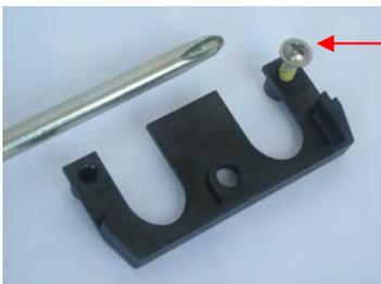
Cut the thread with the screw
