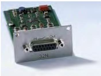
Contact module (catalogue no. LRZ 915) with 15-pole SUB-D socket. Range of functions as LRZ 914, but with three relay contact outputs (changeover, max. 30V/0.2A) and three binary inputs for control via external voltage-free contacts.
