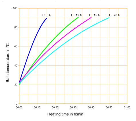
Heat transfer liquid: Water, bath closed
