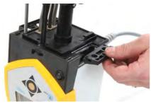
The cooling coil can only be mounted on one side of the control head. This is located on the side with the mains switch.
