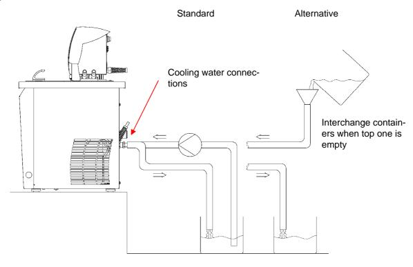
Via the water inlet hose, fill the device with decalcifier (pump or hose). Set the set value to 10 °C; after the chiller starts the water circuit can be filled. Circulate the decalcifier with the pump or continue to top up the decalcifier. Allow the decalcifier to have an effect (see table below). Then drain the device. Again connect the device to the water supply and thoroughly flush it out (see table below).
