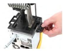
The pump connection set can be mounted on one side of the control head (see illustration).
