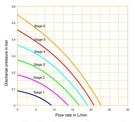
Pump characteristics measured with water
