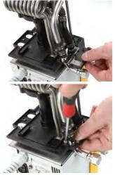
Push the holed flange under the pump connections and fasten it with two cross-head screws to the underside of the control head.
