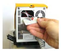
Pull the bus connecting lead out of the plastic cover.
