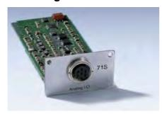
Analogue Module (LAUDA catalogue no. LRZ 912) has two inputs and two outputs, which are brought out to a six-pole DIN socket to Namur Recommendation (NE28).
