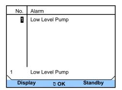
When the liquid level falls so far that the heaters are no longer completely covered with liquid, a two-tone alarm sounds. "Low Level Pump" appears in the display, the heater switches off on all poles and the pump and chiller are switched off via the electronics.
