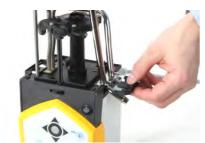
Place the flange of the cooling coil in the position of the removed blind flange and push the holed flange underneath it.
