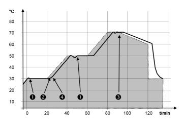
The tolerance entry can have a large effect with external bath control. The adjacent graph of the edited trace shows the possible run-on of the actual temperature in the bath vessel (continuous line) for the set-point temperature of the programmer (highlighted in gray).
