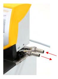
To ensure the greatest volume flow, with operation as a circulation thermostat ensure the shortest possible hose connections with the largest possible hose internal diameter.
