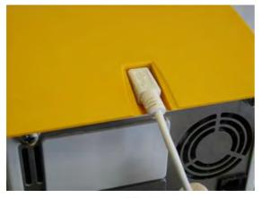
1. Plug the USB cable into the control head.
