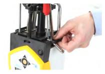
With the two cross-head screws, mount the carrier plate of the cooling coil and the holed flange to the underside of the control head.
