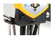
The position **EXT** gives the greatest flow in the external circuit. With the position **INT** the external flow is throttled to a minimum and the outlet for the internal bath circulation is fully opened.
