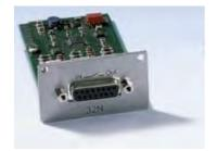
Contact module (catalogue no. LRZ 915) with 15-pole SUB-D socket. Range of functions as LRZ 914, but with three relay contact outputs (changeover, max. 30V/0.2A) and three binary inputs for control via external voltage-free contacts.
