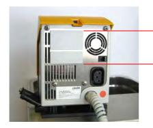
Upper module receptacle (approx. 51 mm x 27 mm) for RS 232/484 module / analog module / contact module / Profibus module
