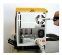
The plastic cover has a recess on each side to ease removal.
