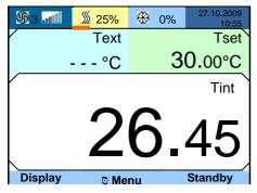
The current bath temperature  $(T_{int})$  is displayed with the status display above it, the expanded status display at the top margin and the soft-key bar at the bottom margin.
