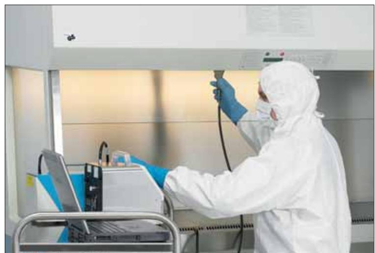
*Testing of the HEPA recirculation filter.*
