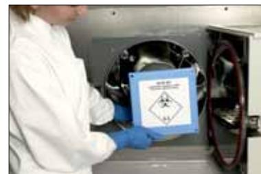
Autoclaving of a HEPA filter cartridge **Best-Filter-Protection**.
