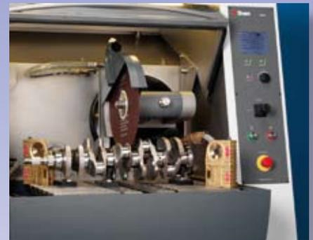
**Axitom-5 is designed for 350 mm / 14" dia. cut-off wheels, equipped with a powerful motor, 2 automatic cutting tables and the advanced ExciCut feature. All functions are controlled by only two keys, making operation extremely user-friendly.**
