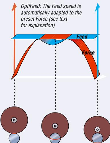
OptiFeed is ideal for cutting of workpieces with varying cross-sections or heterogeneous composition. Variations in such workpieces might otherwise require frequent changes in the feed speed setting and as such pose a problem to many operators.
