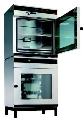
The direct contact between the load and the heatable and removable thermoshelves in the chamber of the Memmert vacuum oven ensures rapid and uniform temperature control of food, cosmetics, watches, books, PCBs or injection moulds, without the loss of heat.
