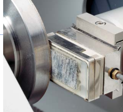
Grinding with cup-wheel on Accutom-50
