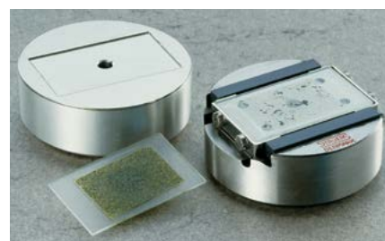
Thin section holders for lapping and polishing
