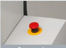
Emergency stop for immediate stopping of all moving parts in case of an emergency
