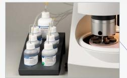
**Dosing module\*** 3 different dosing modules for automatic dosing of consumables
