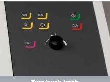
Turn/push knob facilitates and speeds up the entire machine operation and programming
