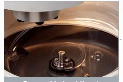
**Removable bowl liner\*** easy cleaning with a bowl liner that collects all debris that is not washed down the drain
