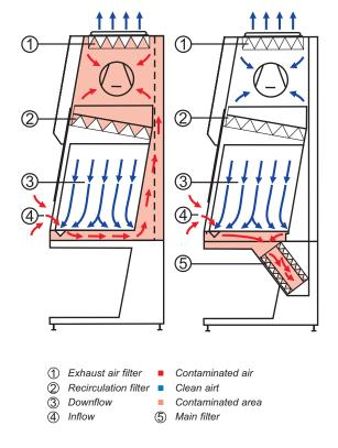
Good things come in three: The patented 3-filter system of the cytostatic safety cabinet **BERNER** Flow**Safe**® has treble the value for you.
