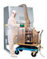
$H_2O_2$  fumigation of a **BERNER** Flow**Safe®** safety cabinet with the SKANAIR® DECOSIS system
